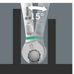
The Joker 6003 combination wrench with its special mouth geometry – an open-end offset by 7.5° and the double hexagon profile – doubles the placement possibilities when repeatedly turning the wrench 180° around the longitudinal axis. Bolts and screw heads can be "accessed" every 15°. The
