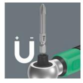
The Safe-Torque A 2 torque wrench has a ¼" bit mounting with a strong permanent magnet and is suitable for bits with ¼" external hexagon drive as per DIN ISO 1173-C 6.3 and E 6.3 and Wera connection series 1 and 4.
