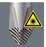
A precisely-focused laser creates a sharp-edged surface structure. This laser treatment results in an edge hardness of up to 1000 HV 0.3. Wera Lasertip "bites" itself into the screw head and prevents any slips out of the recess.
