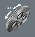
The integrated ratchet with fine toothing (80 teeth) and a return angle of 4.5° eases and accelerates screwdriving without having to reposition the tool.
