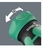
Intuitive switching of the ratchet mechanism. Turn the switch clockwise for clockwise screwdriving; turn it counterclockwise for counterclockwise screwdriving. Use position 0 to deactivate the ratchet mechanism for precise working.
